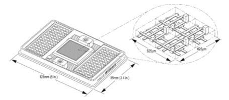
Schematic of our 96.96 Dynamic Array chip including an enlarged section showing four of the chip's 9,216 test chambers.
