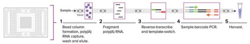
The 48.Atlas<sup>™</sup> IFC architecture automates multiple workflow steps otherwise performed manually, including poly(A) RNA capture, RNA fragmentation, reverse transcription, sample-barcode PCR and multiple wash steps.
