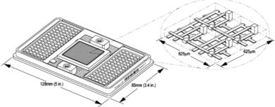
Schematic of our 96.96 Dynamic Array IFC including an enlarged section showing four of the IFC's 9,216 test chambers.
